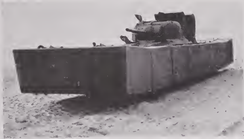
FIGURE 2. Front view of M-4 A1 medium tank equipped with Ritchie T-6 flotation device.
